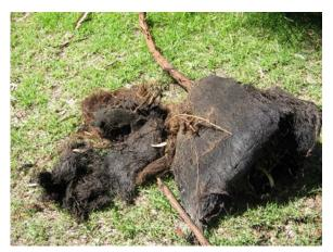
This is a picture of tree roots that had grown in a pump chamber and actually prevented the pump from working. This caused the effluent to back up into the house.
