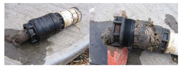
This is a photo showing a build up of sanitary products and nappies jamming both valves in the pump ultimately causing the pump to burnout beyond repair. The cost to replace this pump was taken from the maintenance fund for the respective CWMS.
