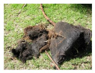
This is a picture of tree roots that had grown in a pump chamber and actually prevented the pump from working. This caused the effluent to back up into the house.
