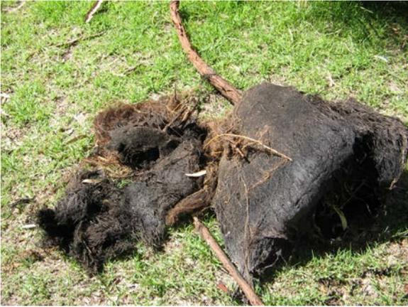
This is a picture of tree roots that had grown in a pump chamber and actually prevented the pump from working. This caused the effluent to back up from the septic tank and into the house.
